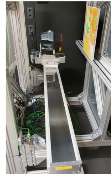
Initial testing of the CAS prototype using mock-up paintings.
